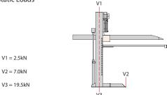
Static load calculations include a vehicle of the maximum weight (2700kg)
